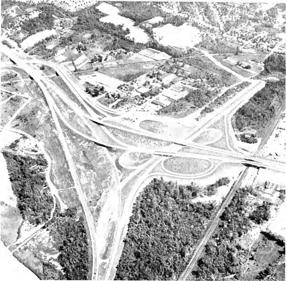
The Baltimore-Washington Expressway connects at its southern terminus with the Kenilworth Interchange, Maryland's most complex grade separation structure.
